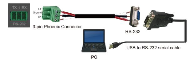
**Step 2.** Check "COM" on the Connection page, and select the corresponding COM Port and Baudrate (default Baudrate: 115200). Then click "Confirm" to connect the device.
