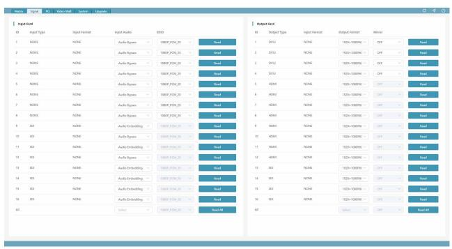
This page is mainly used to configure the relevant parameters of the I/O card.
