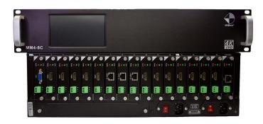
MM4-8C multi-format modular matrix is a HD video and audio signal management device support flexible Video I/O configuration with max 6 video inputs or min 2 outputs configuration. The flexible configuration for the matrix as below: 6In\*2Out/1In\*7Out/4In\*4Out/1In\*1Out/2In\*3Out or more collocation format. The units will support the HDMI/ DVI/ DP/ VGA/ YPbPr/ HDBT/ CVBS/3G HDSDI video format. With scalar output cards the system also will support seamless switching.
